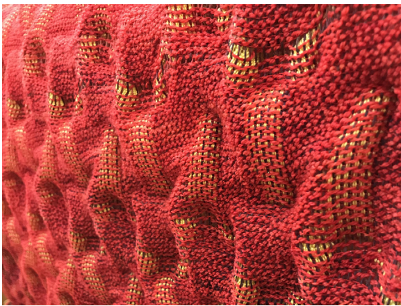
Fig. 3. A three-layer fabric with differential shrinkage and tie-downs in a chevron formation, resulting in a repeating pattern of surface texture.
