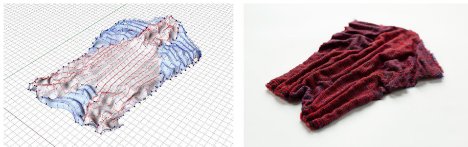
Fig. 17. Modeled surface and fabric panel woven using weaving strategy 3.
