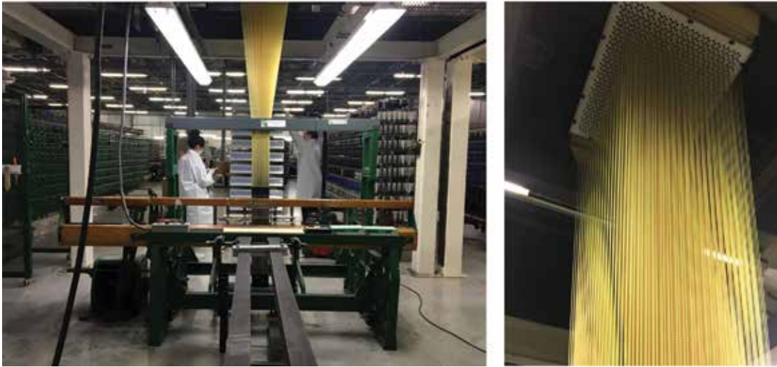
Fig. 3. 3D-weaving loom and castout: industrial Jacquard loom for 3D weaving with creel and detail of harness. (Courtesy of T.E.A.M., Inc., Woonsocket, RI. Photo: Emily Holtzman.)
