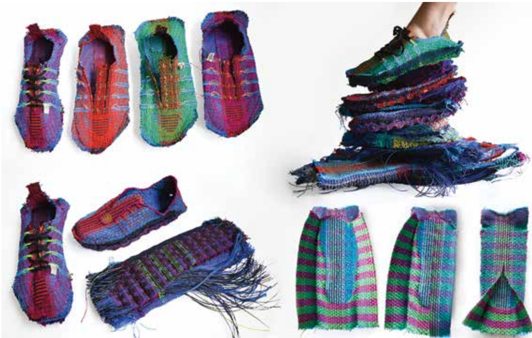
Fig. 9. Iterative process: various shoe versions, following removal from loom; following postproduction finishing; separation of tongue and heel; insertion of laces. (© VTRG 2019. Photo: Emily Holtzman.)
